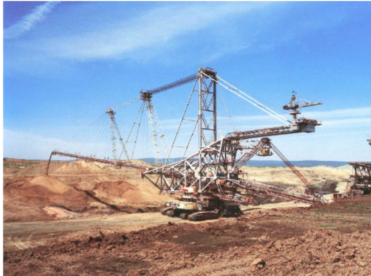
Figure 1: The largest manufactured spreader, produced by TAKRAF, discharge boom length of 195 m, spreading capacity of 8,800 m 3 /h. [13]
