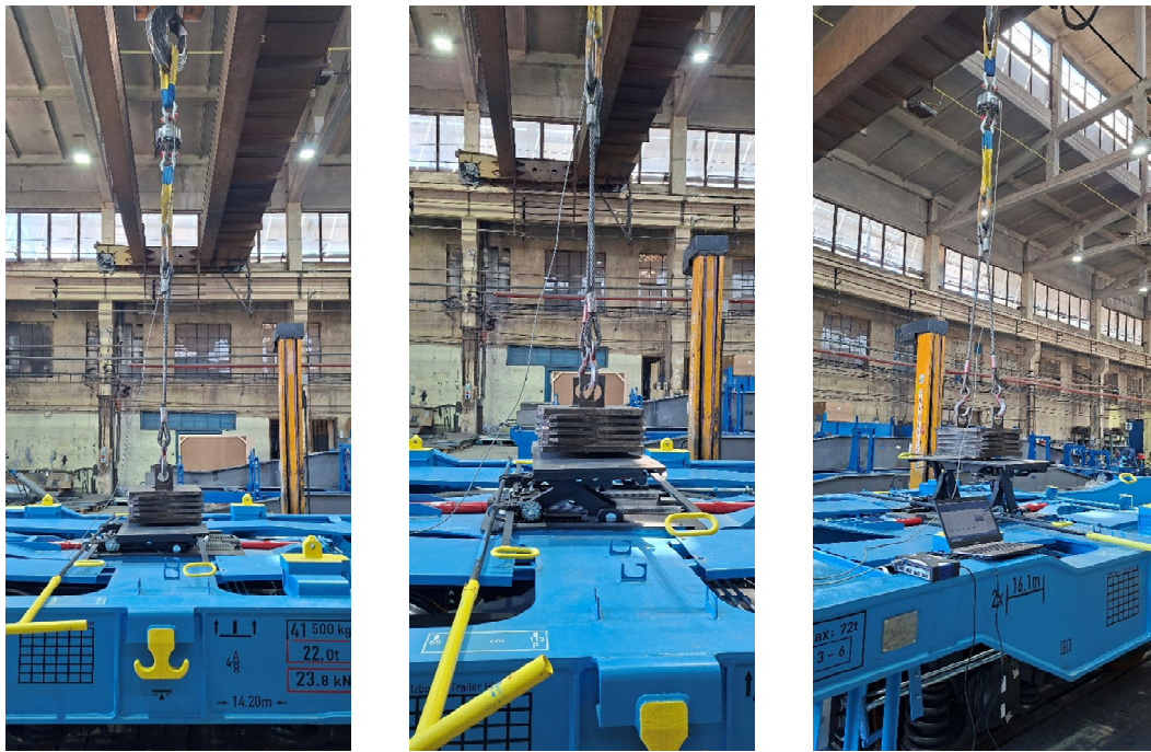
Figure 4: Hitch positions during testing (880, 980, 1130 mm) [9]
