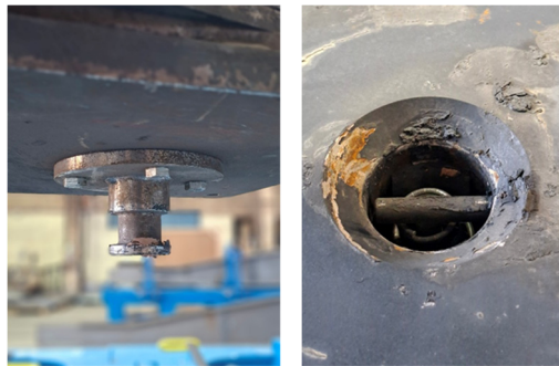
Figure 8: Kingpin and locking mechanism after testing –no visible damage [9]
