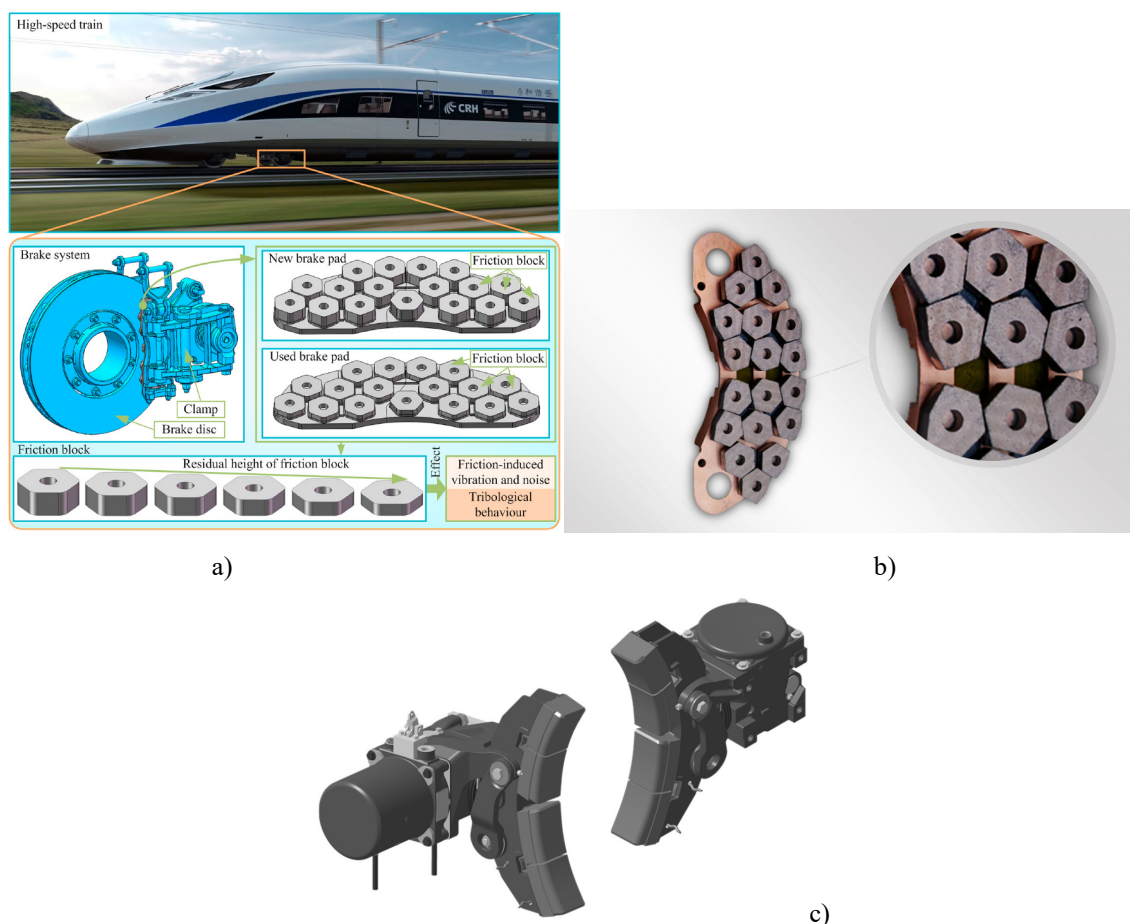
Figure 2: High-speed train disc and tread brake pad [7]
