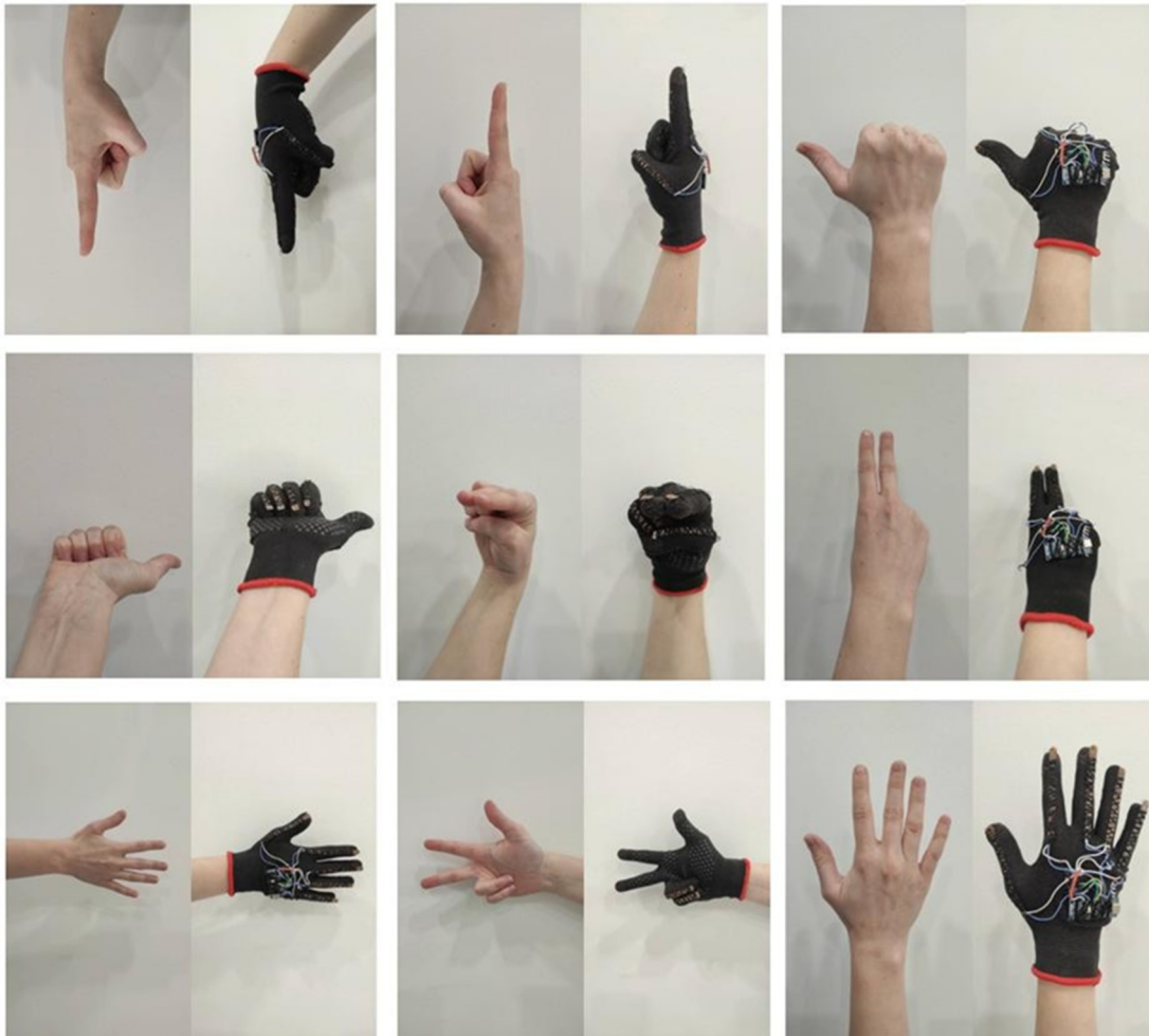
Figure 8: Defined hand commands (down, up, left, right, backward, forward, right rotation, left rotation, stop)
