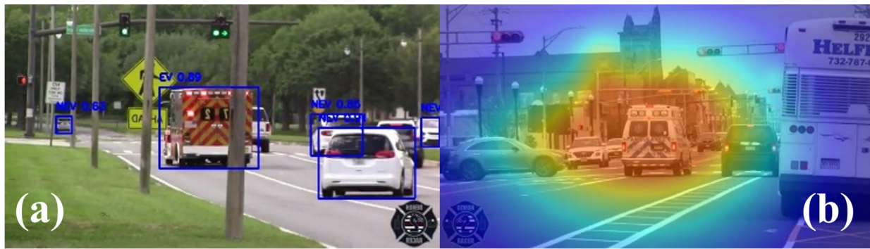
Figure 5: (a) YOLO model annotated emergency and non emergency vehicles and (b) Grad-CAM generated heatmap illustrating key decision-making regions [17]
